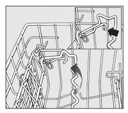
Pull the rail upwards and click it back into position at the required height.
